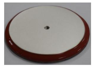
Figure 22. Housingless welding diodes.
