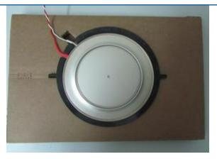
Figure 37. Disc thyristor in internal packaging.
